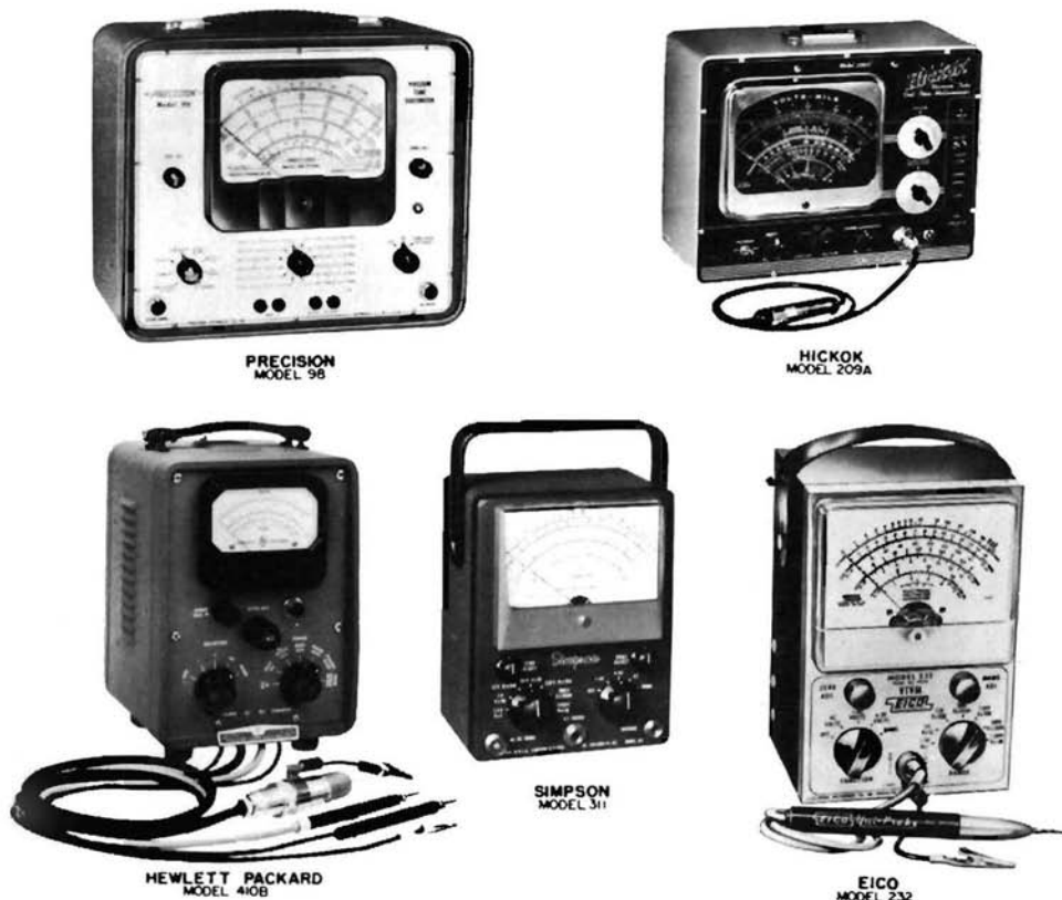
Fig. 10-3. Photographs of typical, modern vacuum-tube voltmeters. (Note: The above photos are reproduced through the courtesy of the manufacturers indicated.)
