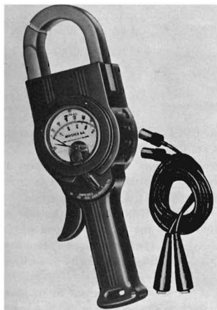
Fig. 6-13. "Clamp-on" type ommeter: (A) Multi-scale volt-meter, Weston; (B) schematic representation of the transformer action of clamp-on ammeter with the wire carrying the measured current acting as the primary.
