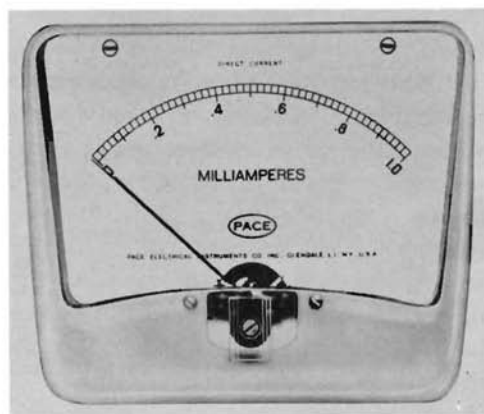
Fig. 1-4 The linear scale used with a typical moving-coil meter (0-1 ma). Pace Elec. Inst., model 45P, (clear acrylic case)
